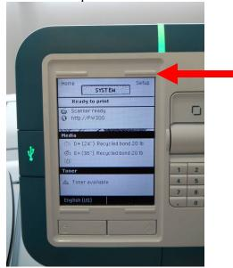
**3.** Use the scroll knob on the right hand side of the interface and scroll down to "Service Info" and press the enter key above the scroll knob on the user interface.
