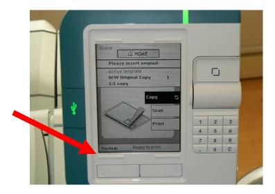
**2.** In the "System" menu press the button at the top right corner directly above "Setup."
